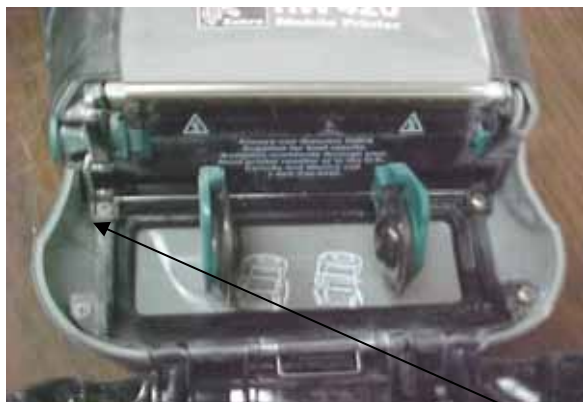
Inspection of Test Unit -Traces of Dust Found →
